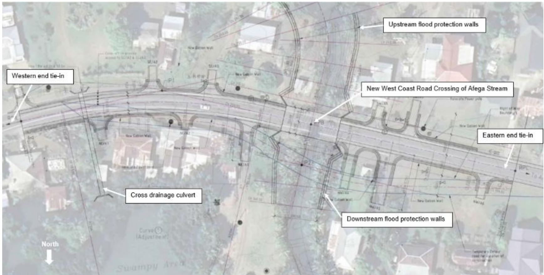
Figure 4: Key features of the replacement bridge
