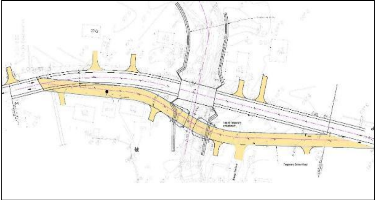
Figure 3: Temporary Detour Road
